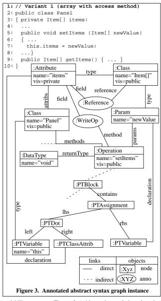
readability reasons. Figure 3 (without the oval-shaped nodes) shows an ASG as an UML-like object diagram, and its corresponding source code.
