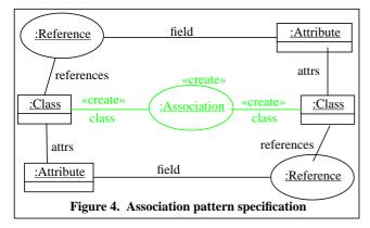
used, the subgraph to be matched in the host graph is defined by the black nodes and edges. The subgraph to be added is defined by the grey node(s) and edges annotated with the keyword "create". This simple notation can be used because the rules only add information to the host graph and never delete any. (The formal definition and theory underlying such graph transformation rules is given in [SWZ95].)
